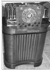
The 1941 EH Scott AM-FM Philharmonic placed Second in both RF and Audio performance. It should also be noted that this 33 tube radio is from 1941 but only the AM was evaluated and it had the recent IF modifications and alignment which corrects the detected distortion problem in all Philharmonics.
