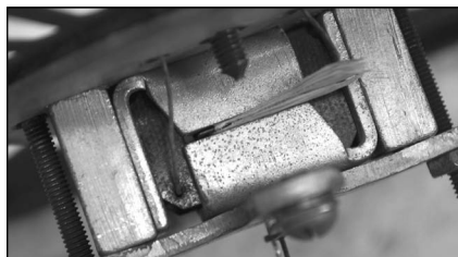
Closeup of the pole pieces showing the iron leaf held in position by paper shims
