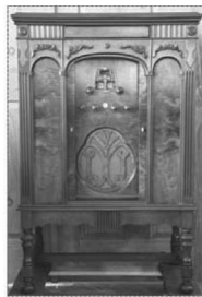
The 1933 McMurdo Silver Masterpiece II ranked Eighth. It was completely disassembled, all metal parts re-chromed and re-assembled and aligned in 2011. The cabinet was originally fitted with the same model II radio and refinished in 2011 too.
