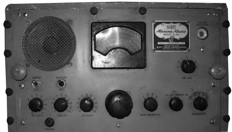
E.H. Scott SLRM Marine Radio – Audio produced by 2 25L6 tubes. Low radiation receiver. Steve Tessler, Detroit, MI.
