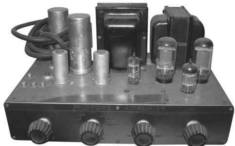
Pilotone Model AA903 – This is an audio amplifier. Uses 2 6V6 output tubes. Runs approximately 15 watts output. Chris Ponce, Austin, TX.
