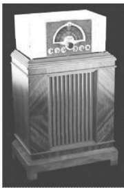
The 1936 McMurdo Silver Masterpiece II ranked Seventh. It was purchased, electronically restored and aligned in 2009. It is completely original with the exception of the cover being re-chromed, it has the re-coned 18" Jensen speaker and Clifton cabinet with the back.
