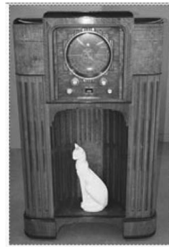
The 1935 Zenith Stratosphere 1000z placed Third. It was rebuilt electronically and the cabinet expertly refinished in 2008 and performs well. It also uses two Jensen A12 and one "Q" tweeter speaker, which were standard for the Stratosphere in 1935.
