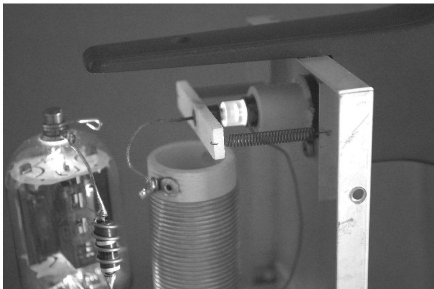
The Ionovac speaker seen in operation.
