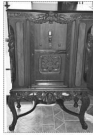
The 1932 EH Scott All Wave 12 Deluxe ranked Sixth. It was completely disassembled, all metal parts re-chromed and re-assembled and aligned in 2010 and placed in a 1930s Philco cabinet, it has the original finish and uses a Jensen A12 speaker.
